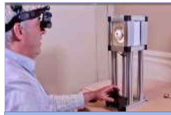
BIObot- showing the use of the joystick to control the direction of gaze
